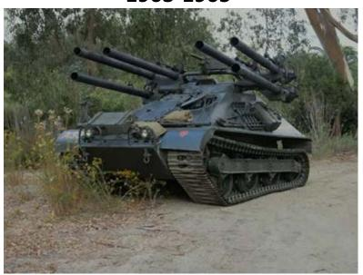
The M50 Ontos (Greek for "Thing") was the weapon of the 1<sup>st</sup> Anti-Tank Battalion. Mounted on the Ontos were six 106 mm recoilless rifles that could be fired in rapid succession or as a salvo against single targets to guarantee a kill.
